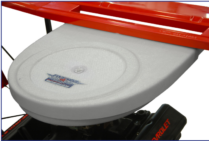
FULLY INSTALLED COLD AIR BOX
