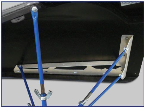
000-500: MOUNT TO INSIDE OF WEAR STRIPS WITH A FIVE STAR UNIVERSAL BODY MOUNTING KIT
