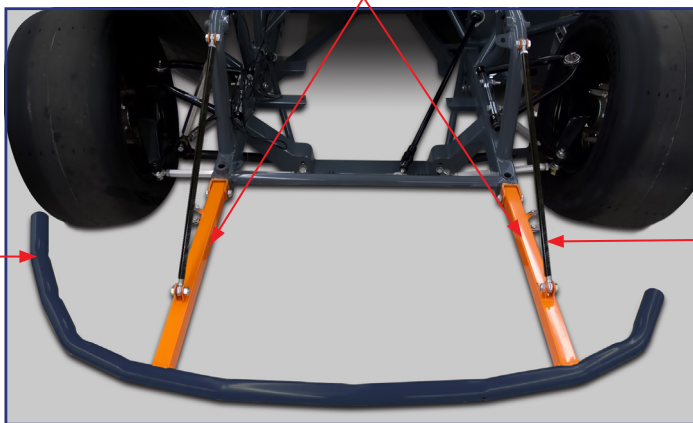
FRONT BUMPER MOUNTING KIT (HIGHLIGHTED IN ORANGE) WITH BLACK ADJUSTABLE BUMPER SUPPORTS
