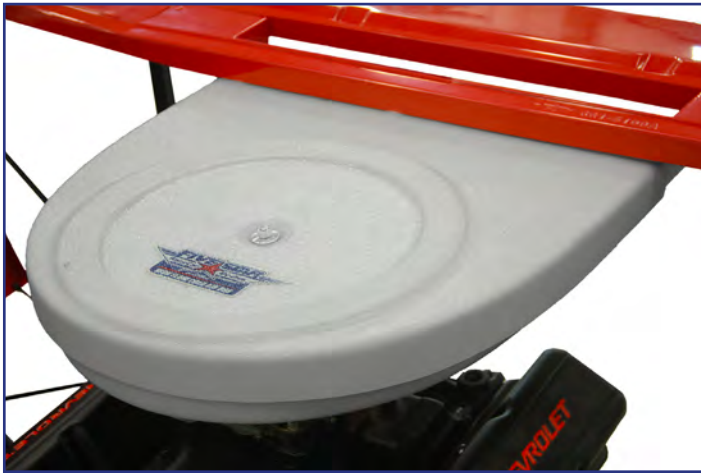
FULLY INSTALLED COLD AIR BOX
