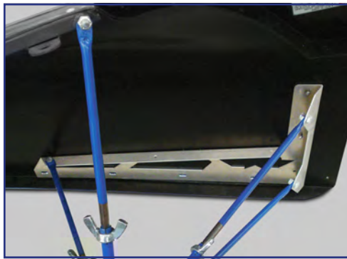
000-500: MOUNT TO INSIDE OF WEAR STRIPS WITH A FIVE STAR UNIVERSAL BODY MOUNTING KIT
