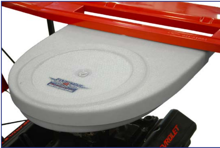
FULLY INSTALLED COLD AIR BOX
