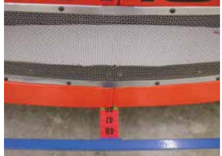
Front overhang is measured by viewing the gauge at the base of the nose.
