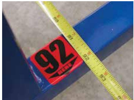
The 92 inch dimension is critical to ensure tread width gauges are properly calibrated.
