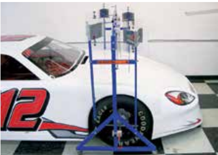
Insert left side tread width measuring arm into left wheel and lock into place. Repeat this procedure on the right side.
