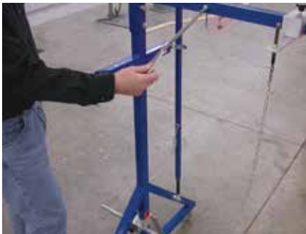
Adjust hex rod to obtain 92 inches from outside to outside of device.
