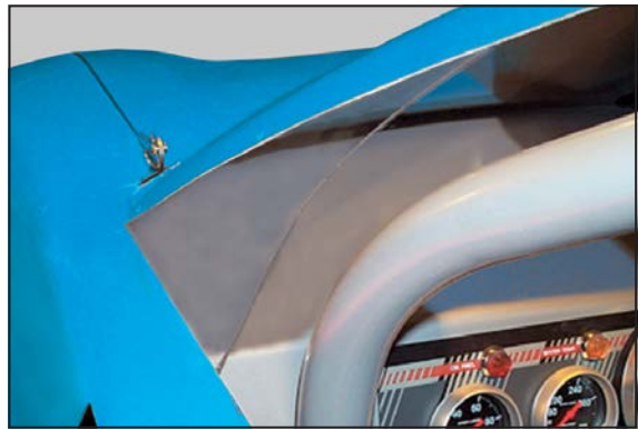
THE 000-6202 DOOR VENT WINDOW IS OVERSIZED; TRIM TO FIT YOUR APPLICATION
