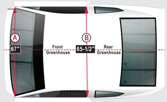
Note: The Front Roof Height is measured 10" back from the windshield, on the centerline.
